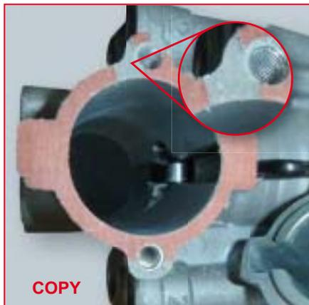
The missing sealing material in the copy part increases the risk of water and dirt getting in.
