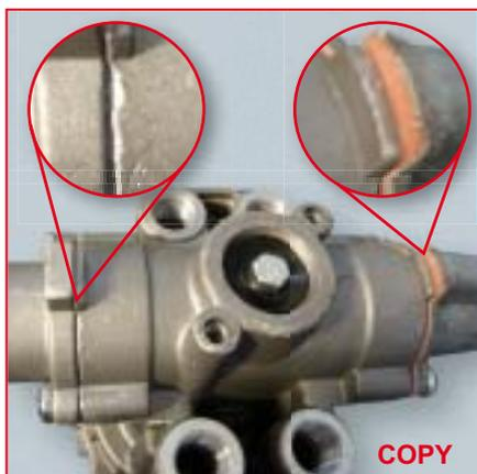
The deformed edges of the housing and housing components that do not close completely encourage leakage.
