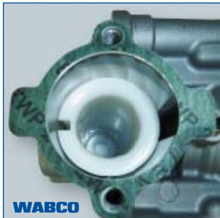
This can mean that the load pressure is no longer being recorded correctly and ultimately the vehicle will no longer brake according to its load. With a light load, this may cause the wheels to lock because there is too much braking pressure. With a heavy load, on the other hand, the braking force will be inadequate - in both cases this will increase the braking distance in an uncontrollable way, causing a critical safety situation.
