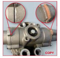
The deformed edges of the housing and housing components that do not close completely encourage leakage.
